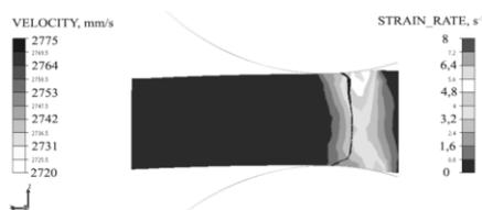
Fig. 7. Distribution of strain rate intensities  $\dot{\epsilon}_i$  for feedstock of an initial height of  $h_0=200$  mm, rolled with a reduction of  $\epsilon=0.10$ , with an asymmetry factor of  $a_v=1.00$ , and at a deformation zone feedstock feed angle of  $\theta=3^\circ$
