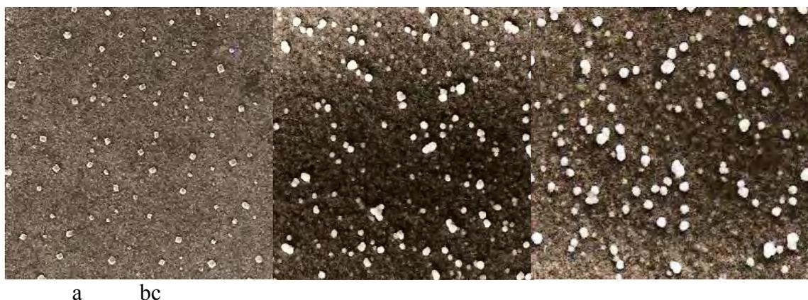
Fig. 2. Microphotographs of composite sediment on nickel substrate. Containment of nano-fraction powder mixture (g/l): a) bentonite – 2; b) caolinite – 2; c) bentonite – 1, caolinite – 3
