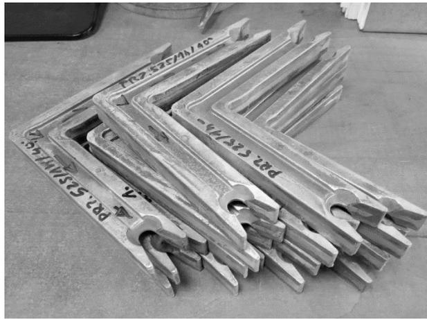
Fig. 13 Forged connectors made from aluminium alloys series 6005 and 6082
