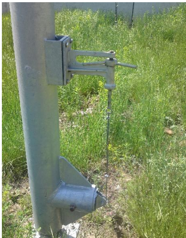
Figure 3.11 - Hand brake of the wind turbine.
