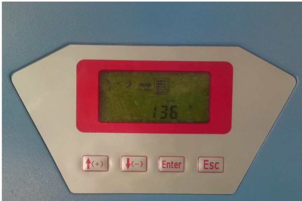
Figure 3.13 - Control panel on the wind power panel.
