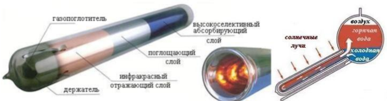
Figure 3.31 - Composition and operating principle of vacuum tubes.
