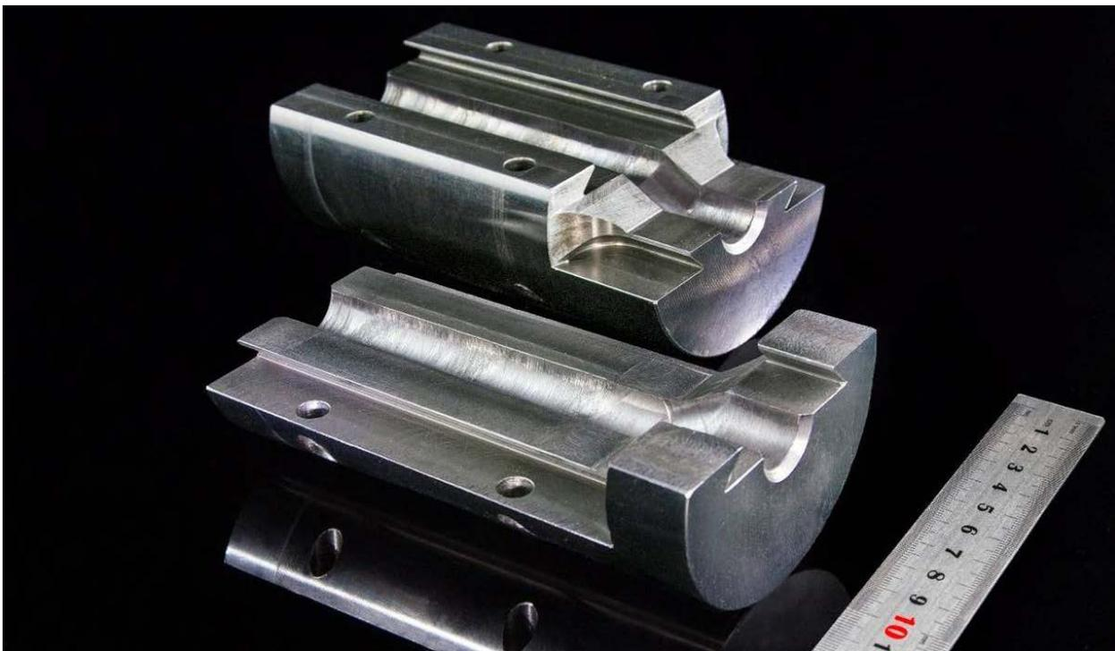
Figure 5.10 – Fabricated matrix with a channel diameter of 18.5 mm
