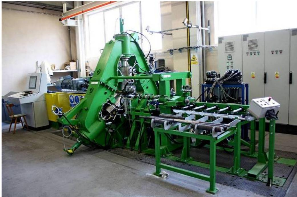
Figure 7.4 – Experimental-industrial mill MMV
