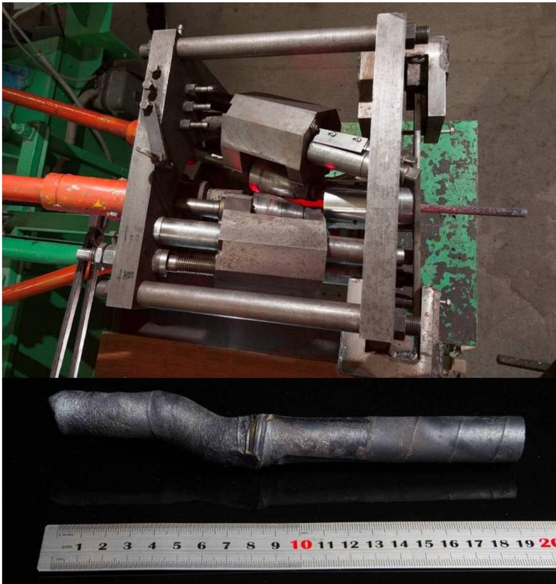
Figure 5.15 – Stand of the combined process "screw rolling-pressing" at the time of commissioning and under-rolled billet
